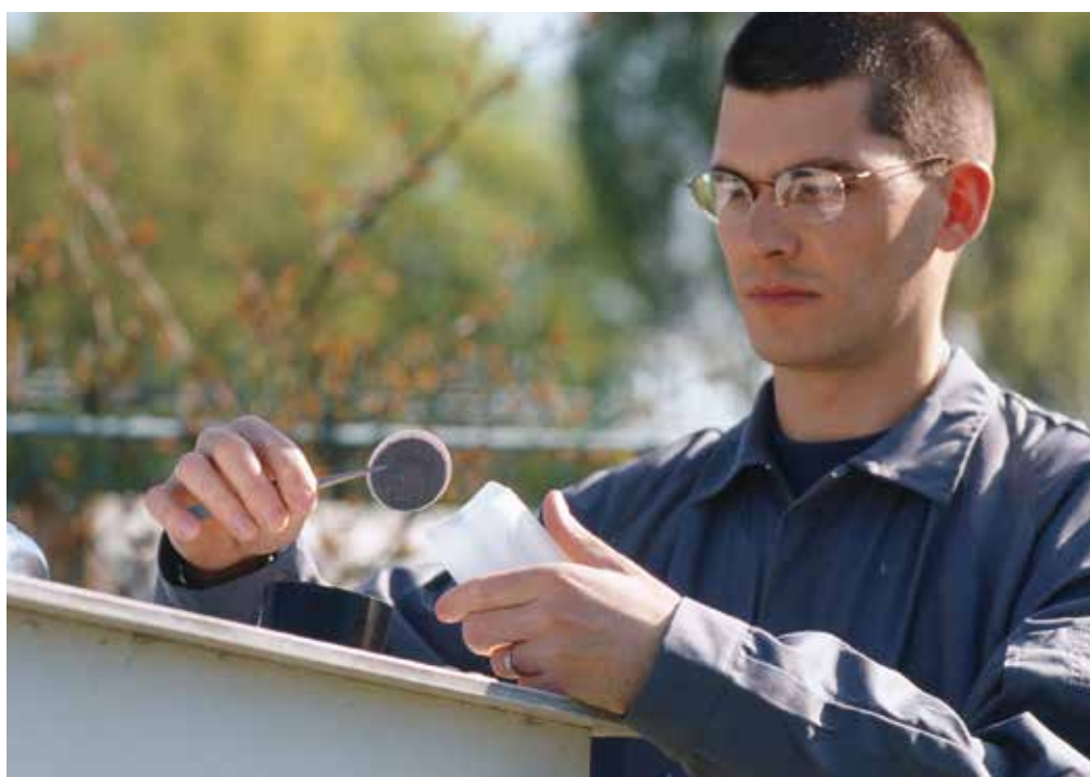
Taking samples using an aerosol filter
