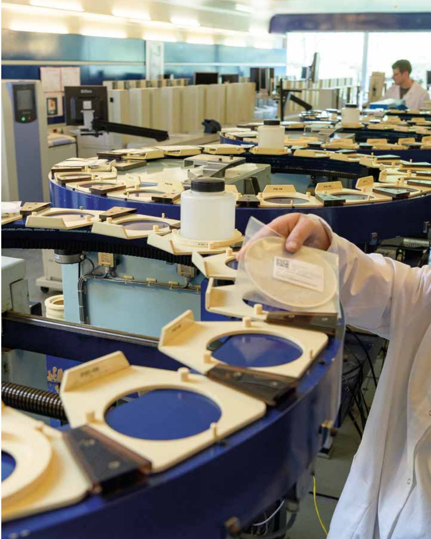
Gamma spectrometry system for measuring atmospheric aerosol filters
