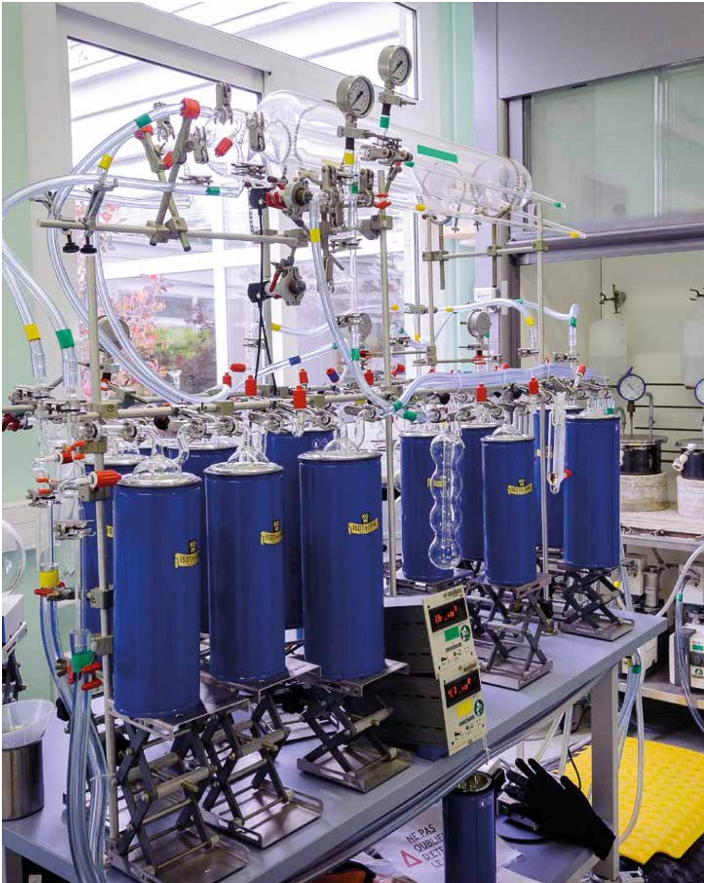
Carbon-14 measurement bench based on benzene synthesis
