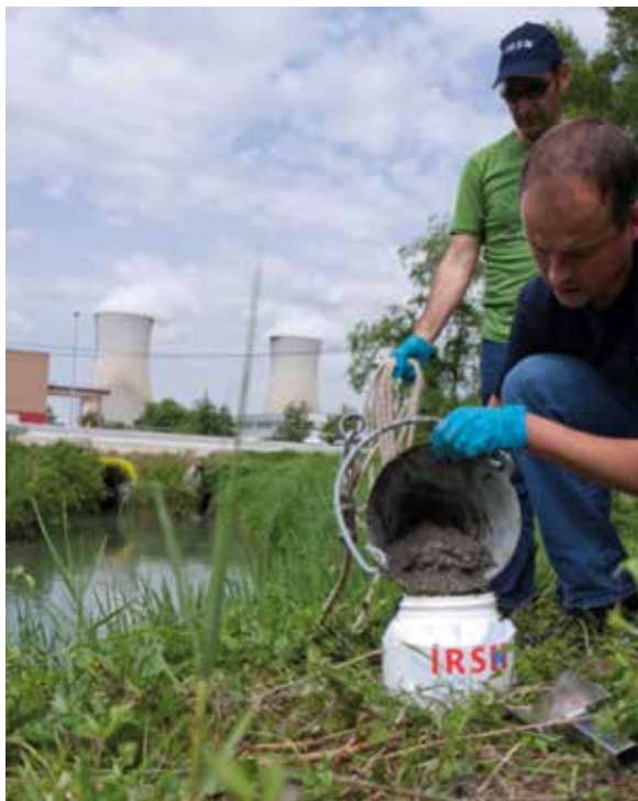
FIGURE 10 / AD HOC SEDIMENT SAMPLING USING A BERTHOIS CONE
