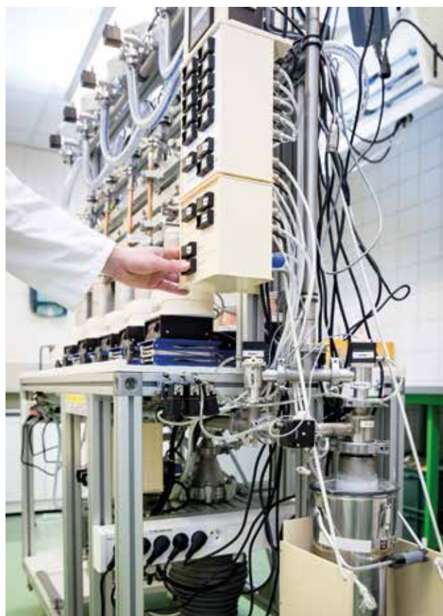
Helium-3 degassing bench for seawater tritium measurements
