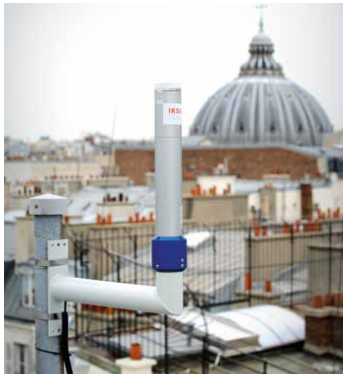
FIGURE 1 / AMBIENT GAMMA DOSE RATE CONTINUOUS MEASURING SYSTEM, PART OF THE IRSN TÉLÉRAY NETWORK (photo 1A) AND RPL DOSIMETER SET UP AT THE CADARACHE SITE (photo 1B)
