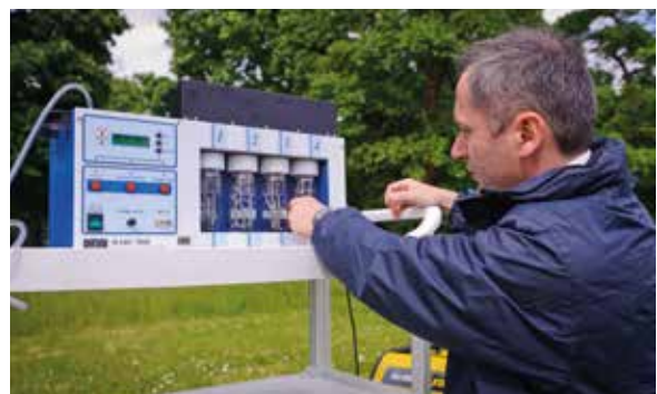
FIGURE 4 / BUBBLERS FOR TAKING ATMOSPHERIC TRITIUM OR ^{14}C SAMPLES
