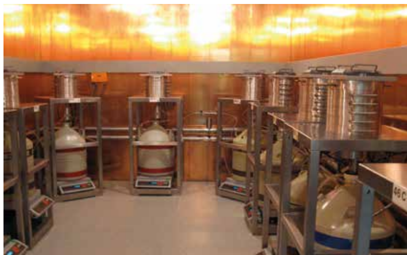
IRSN's gamma spectrometry room at Orsay can be used to measure very low activity levels
