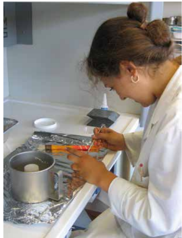
Crushing and adjustment of the geometry of a dried grass sample
