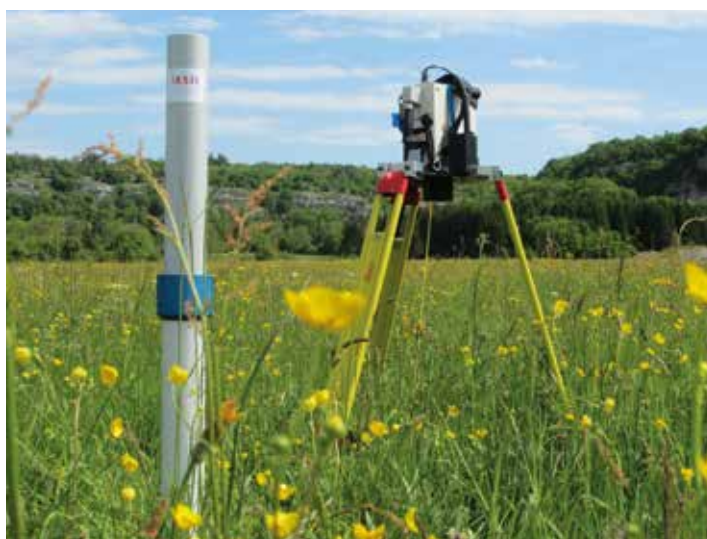
Téléray sensor (left) and field gamma spectrometry system (right)
