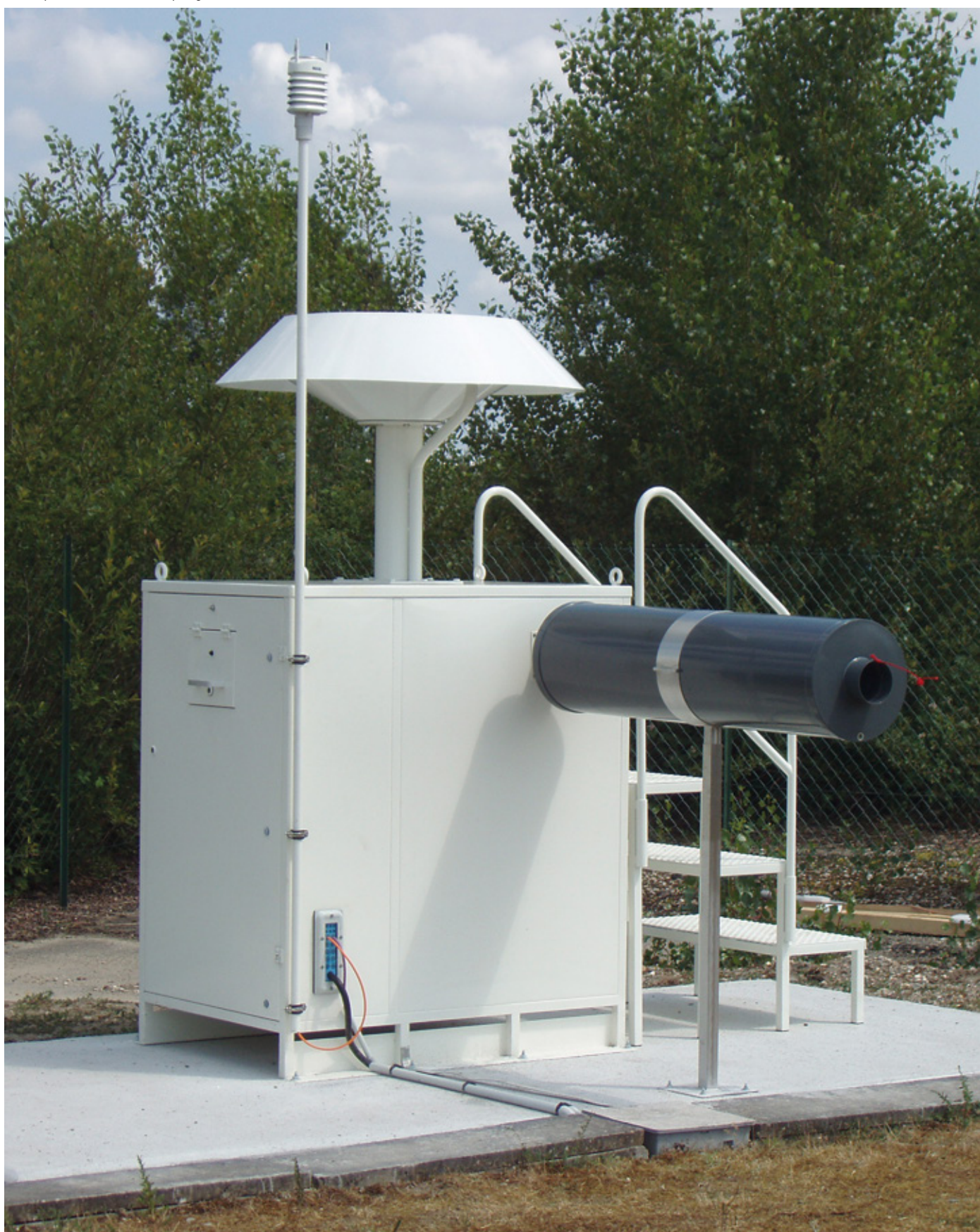
Atmospheric aerosols sampling station OPERA-AIR TGD 700 m 3 /h
