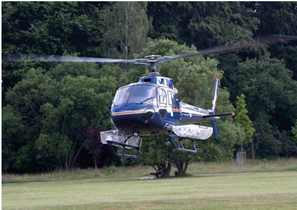
IRSN's Ulysse onboard gamma spectrometer; the sensors are installed in the pods on each side of the helicopter. This set-up was used, on a plane, to obtain the data shown in the map in figure 5A.
