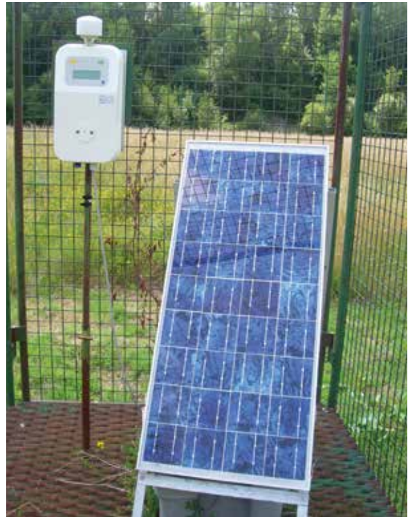
FIGURE 4 / BUBBLERS FOR TAKING ATMOSPHERIC TRITIUM OR ^{14}C SAMPLES
