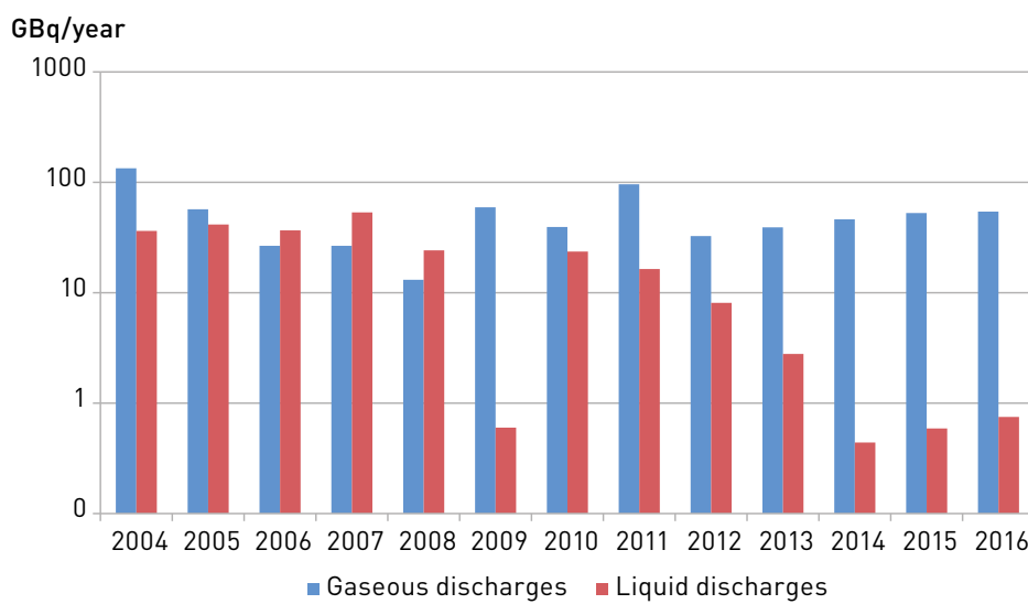
FIGURE 2 / VARIATION IN LIQUID AND GASEOUS TRITIUM DISCHARGES FROM THE CEA SITE AT CADARACHE SINCE 2004 (GBq/year)
