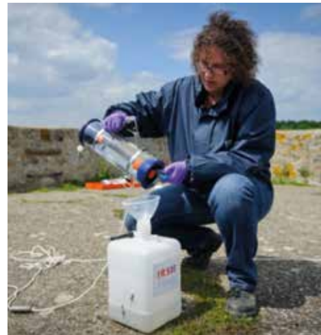
FIGURE 9 / AD HOC WATER SAMPLING USING A HORIZONTAL KEMMERER SAMPLER
