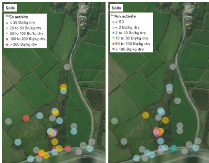
FIGURE 5 / ACTIVITY RANGES OF CAESIUM-137 AND AMERICIUM-241 MEASURED IN THE SOILS (Bq/kg dry)
